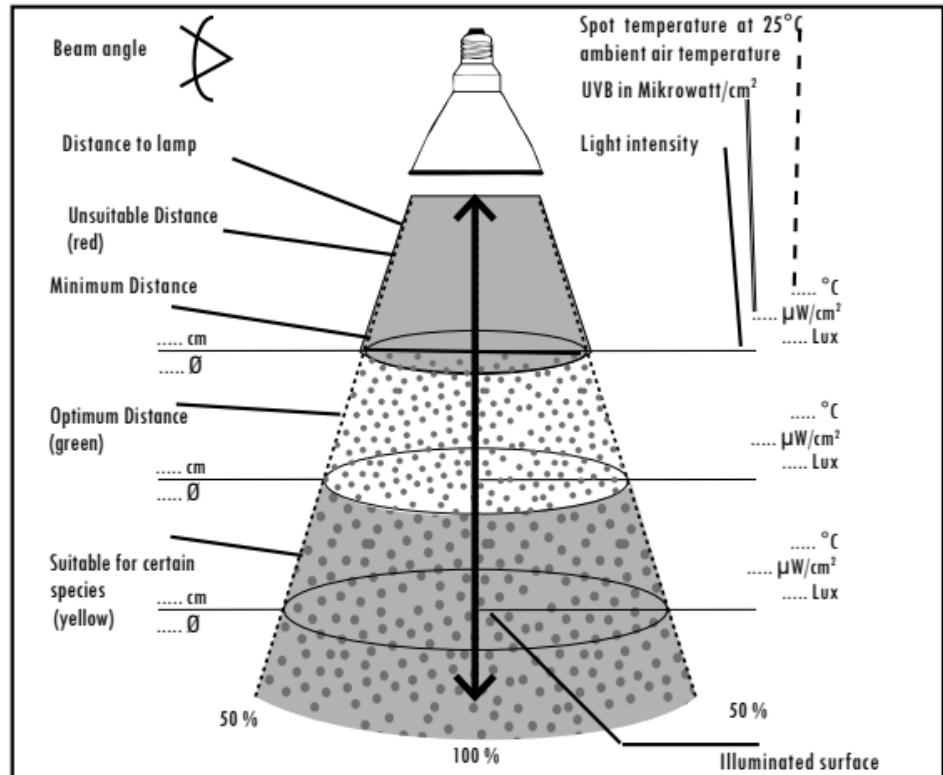
Please consider that the UV amount on the illuminated surface will be heavily dependent on the distance to the lamp. Reducing the distance by half will quadruple the UV amount and vice versa. At 20 cm the UV performance is 4 times higher than at 40 cm. For this reason you should consider our distance recommendations for the safety of your animals.
